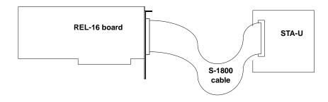
Figure 1. Connecting an REL-16 Board to an STA-U
