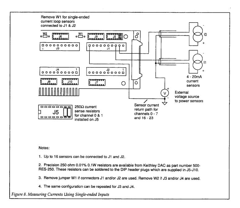
common current return is used as shown for single-ended current inputs, single-ended voltage inputs in that group of 16 cannot be used. Figure 9 shows a single 4-20 ma sensor connected up for current sensing in the differential mode. In this connection method, either input terminal on the AIM3A may be connected to ground either at the external power supply or at the sensor.
