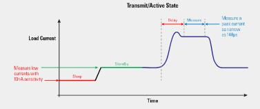
The Series 2280S can make fast current measurements on a load burst that is as narrow as 140µs and can easily monitor load currents during all operating modes of a device to determine its total power consumption without the need for extra equipment.
