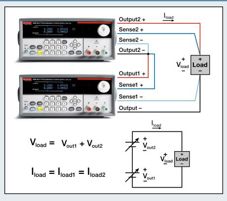
Use several supplies or combine the outputs in a multiple output supply to increase output voltage or current. For multiple output supplies, ensure that all the outputs are isolated; that enables the channels to be combined in either series or parallel. Keithley's multiple output power supplies provide features to simplify controlling and displaying the voltage and current when outputs are connected in series or parallel.
