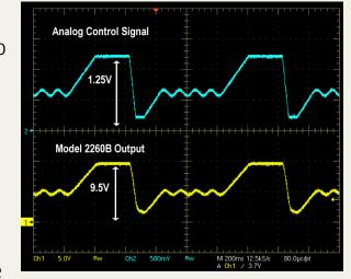
of voltages. They have variable slew rates to create rise and fall conditions. Some models have analog inputs to enable an AC waveform to be superimposed on the DC line for simulation of a noisy line. Many of these features minimize the test instrumentation needed to thoroughly test a DUT.
