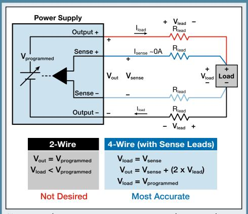
No matter how accurate your power supply output is, you cannot guarantee that the programmed voltage is the same as the voltage at the DUT's terminals. A power supply without sense leads regulates its voltage at its output terminals. However, the voltage you want regulated is at the DUT's power inputs. The power supply and the load are separated by lead wires that have a resistance, RLead; thus, the voltage at the load is:
