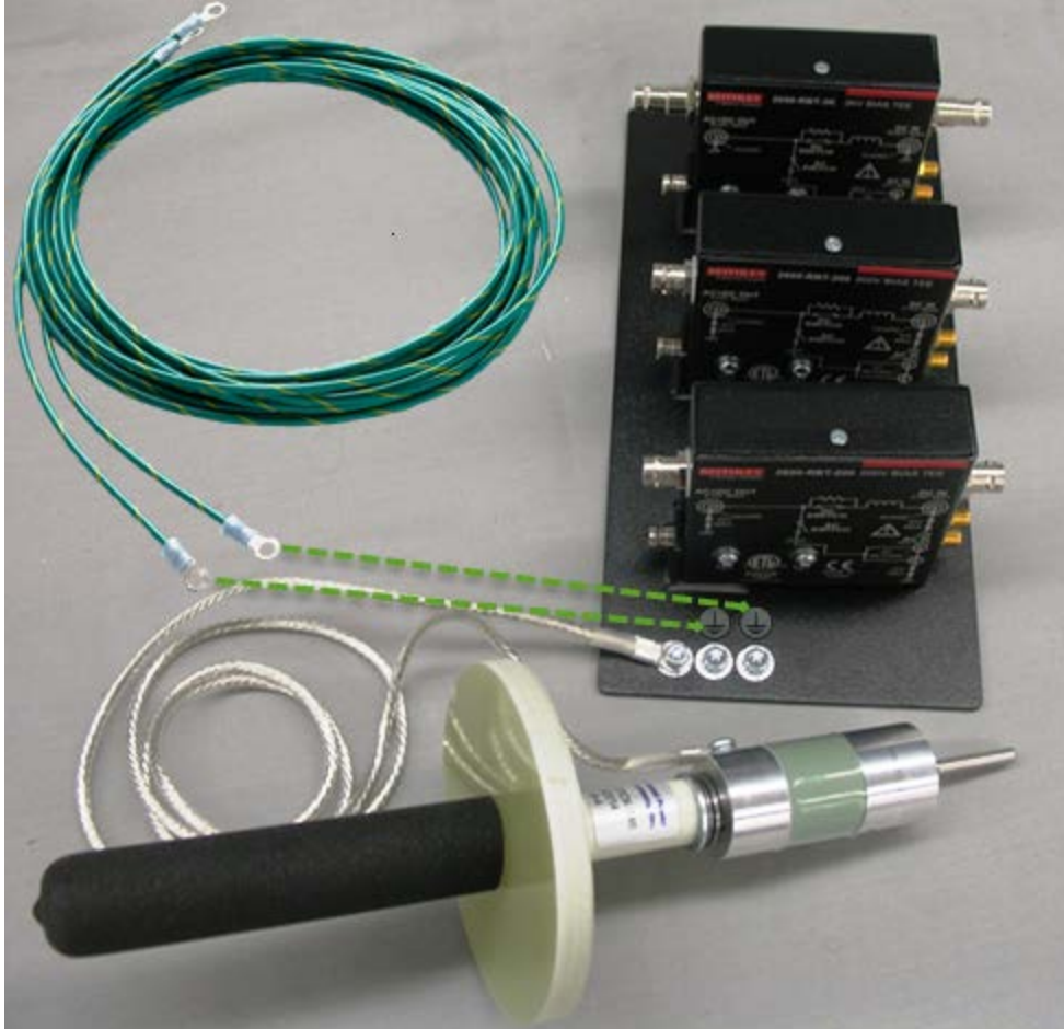
Figure 3: Bias tee mounting bracket with CA-568-120 grounding cable connection
