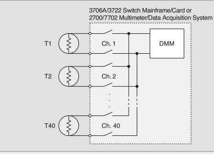
Figure 19. Measuring temperature using thermistors
