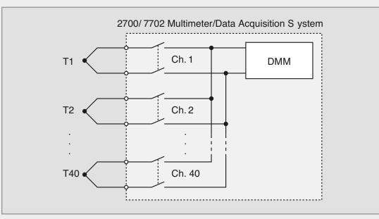
Figure 15. Using simulated reference temperature with the Model 2700/7702
