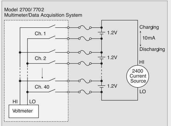
Figure 1. Charging/discharging multiple batteries in series
