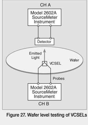
Vertical-cavity surface-emitting lasers (VCSELs) are slowly replacing traditional Measuring the PDs can be done with either a Model 2602A or 2636A,
