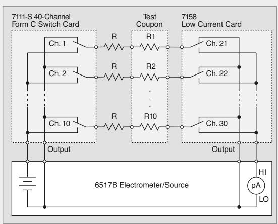
Figure 10. Circuit to test a single ten-resistor coupon
