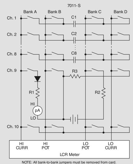
Open-circuit and short-circuit channels are omitted for clarity.
