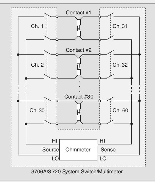
Figure 11. Measuring resistance of 30 contacts
