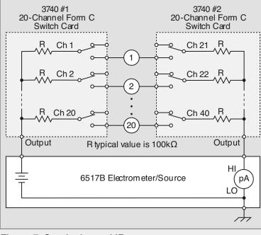
Figure 7. Continuity and IR test system
