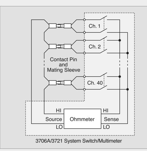
Figure 12. Measuring 96 contacts with a common terminal
