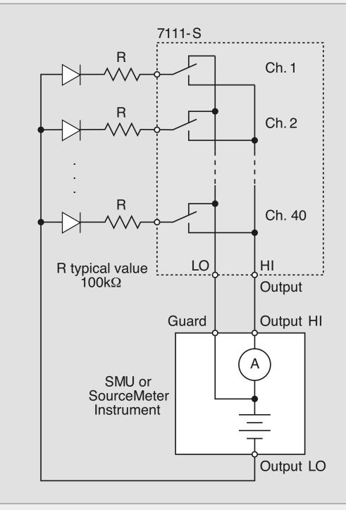
Figure 22. Using an SMU or SourceMeter Instrument to test the leakage current of diodes
