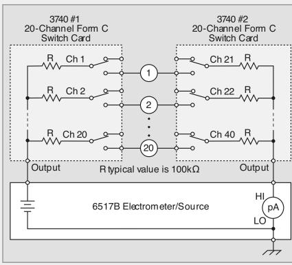
Figure 6. Testing IR between any two terminals
