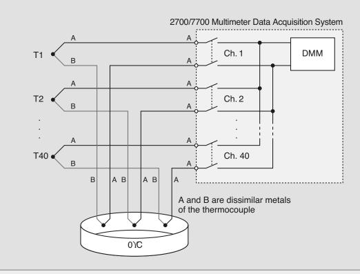
Figure 16. Using "back-to-back" thermocouples and a 0°C reference temperature
