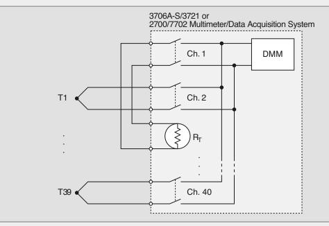
Figure 17. Using a thermistor as an external reference junction
