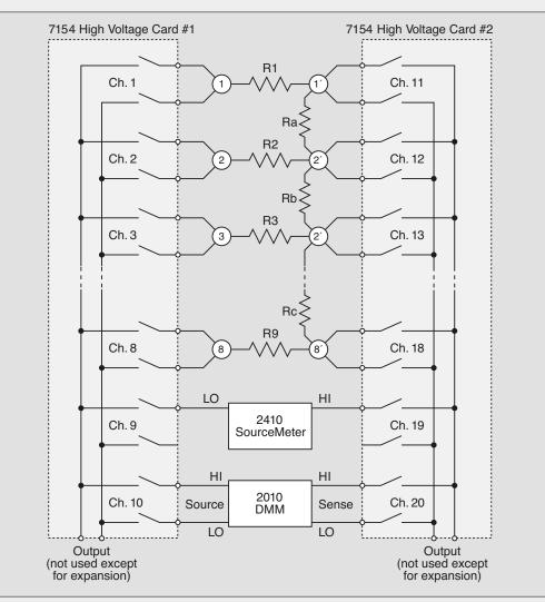
Figure 8. Expanded range continuity/IR system
