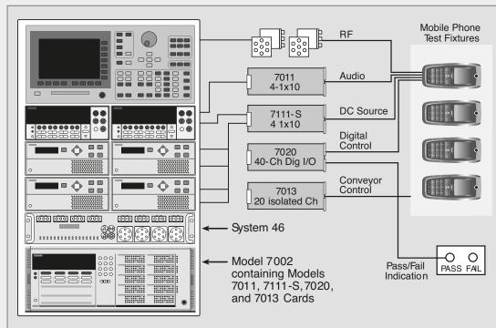
Figure 26. Cell phone test system
