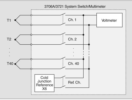
Figure 14. Using the internal reference junction of the Model 3706A/3721
