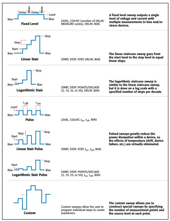
Figure 7. Various sweeps supported by SMU instruments.
