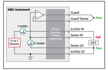
Figure 12. Series 2400 contact check
