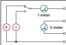
Figure 1. Basic SMU instrument topology
