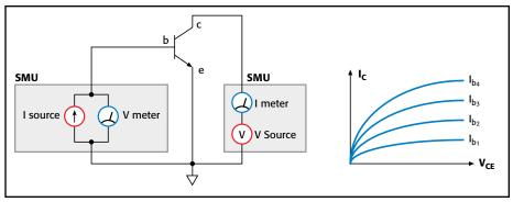
Figure 6. Typical family of curves for transistors
