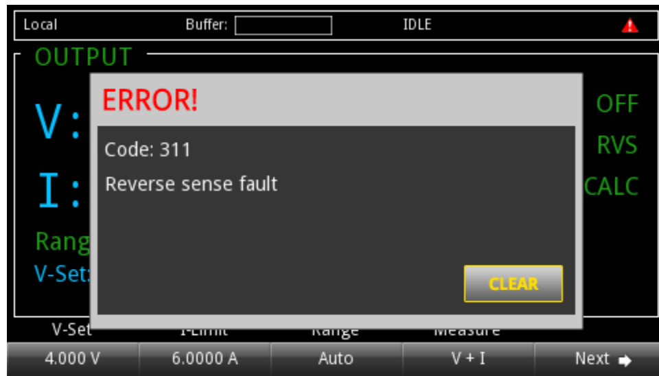
Figure 41: Reversed sense leads error
