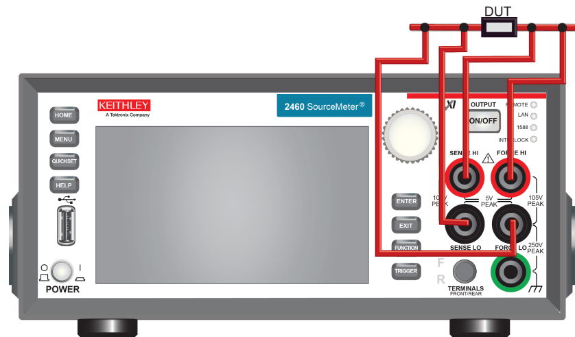
Figure 62: Model 2460 4-wire sense front panel connection
