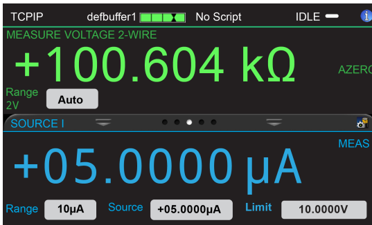
Figure 68: Resistance measurement SIMV SCPI example
