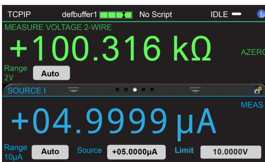
Figure 69: Resistance measurement SIMV and read ohms
