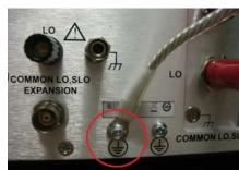
Figure 37: 8020-DP connected to protective ground
