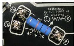
Figure 19: Resistor installed between nodes 1a and 2
