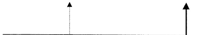
Figure 8-7. Glitch Trigger: here on a pulse width less than or equal to the width selected. The broken upward arrow indicates a potential trigger, while the bold one shows where the actual trigger occurs.
