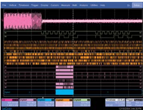
MS-32 extends the range of WaveSurfer and WaveRunner by enabling 4 analog channel and 32 digital channel (4+32) measurement capability.
