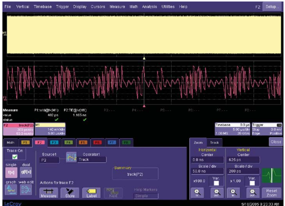
Track of TIE@level is displayed in math function F2.
