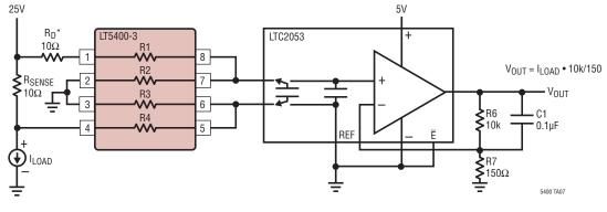
\* -1% VISHAY CRCW1206 AS LONG AS RD-RSENSE << R1 - R4, THE COMMON MODE REJECTION WILL NOT BE DETERIORATED BY THE SENSE RESISTOR.
