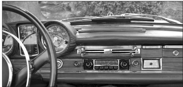
Figure 1. Old school dashboard; one passive antenna for AM/FM reception
