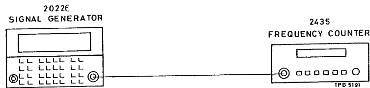
Fig. 5-2 Test gear arrangement to check frequency accuracy
