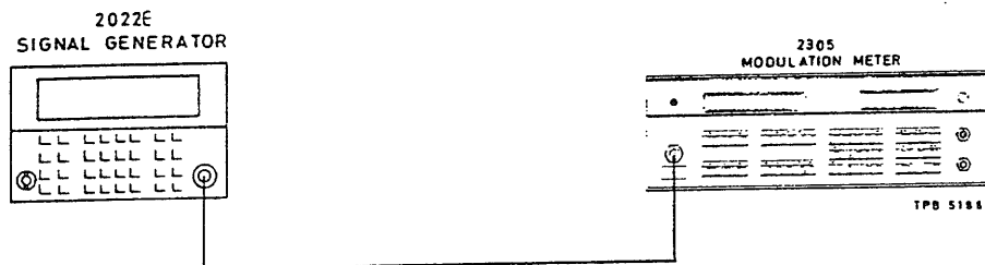
Fig. 5-5 Test gear arrangement to check FM deviation and distortion
