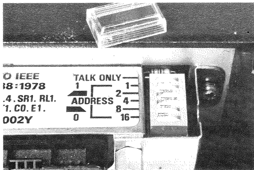
Fig. 2-3 Switches on the 2955's GPIB interface unit set to address 6 (2 + 4) and not to TALK ONLY
