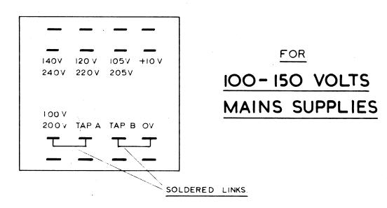
A ARRANGEMENT OF PRIMARY SOLDER TAG CONNECTIONS ON MAINS TRANSFORMER.
