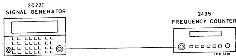
Fig. 5-2 Test gear arrangement to check frequency accuracy
