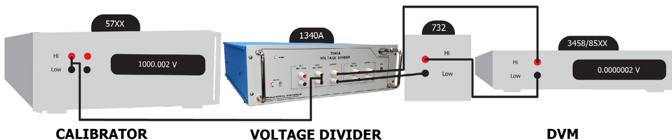
Figure 2. The above diagram illustrates using a 1330A, 732B or 732C reference in the connection sequence. A DVM can be used as a NULL detector to determine the offset of the 57XX series on the 10:1 and 100:1 ratio.
