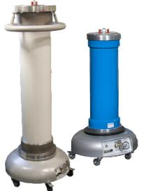
The high voltage capacitors consist of a low voltage measurement electrode which is isolated from the high voltage electrode by a dielectric gas (SF<sup>6</sup>). A guard electrode or grounding technique can be used to eliminate parasitic capacitance. Grounding or connecting the guard circuit are specific to the installation and application.
