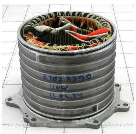
\Drive Motor Asm \Stator Housing Asm \Stator Asm, Stator Housing Asm
