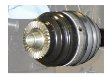
The BMW i3 half shaft assemblies are of the Schaeffler LUK FAG Axial spline design type with unique features which help unit balance and durability including large boot clamps without protrusions and inner race bearing channels with chamfered edges. Weight reduction strategies included tubular shafts, axial spline design and aluminum boot clamps
