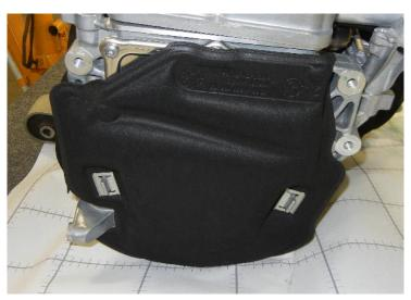
\Zone 7 Driveline \Motor \Thermal Cover Motor Installation
