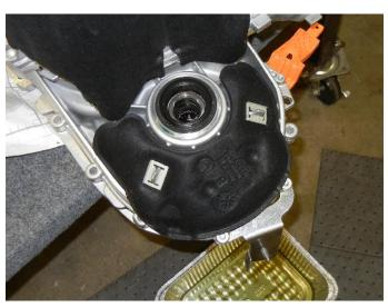
\Zone 7 Driveline \Gear Box \Thermal Cover, Differential Installation
