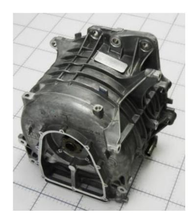
Zone 7 consists of the electric motor, gear box, and half shafts. The electric motor for the i3 is a liquid cooled three phase permanent magnet induction motor. The gear box for the i3 is a single speed fixed ratio design. Half shaft assemblies are Schaeffler LUK FAG Axial spline design with unique features to optimize weight. Assembly and manufacturing details for all three components will be covered throughout the report.
