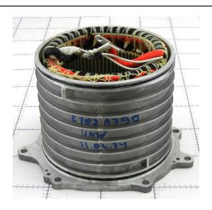
\Drive Motor Asm \Stator Housing Asm
