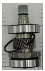
\Gear Box Asm \Parking Brake Gear, Gear Box Asm
