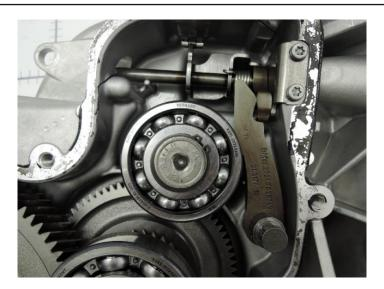
\Gear Box Asm \Gear Box Housing, Gear Box Asm \Assemble Parking Brake Pawl
