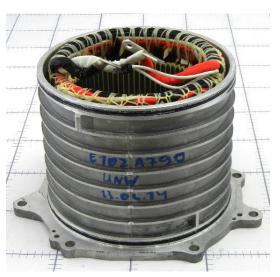
**\Stator Housing Asm** \Stator Housing, Stator Housing Asm **\Stator Housing Process**
