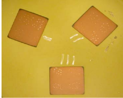
Figure 2. 22 \mu F 25 V capacitors after Vickers hardness testing. Dots indicate marks after indentation testing made at different levels of the load.
