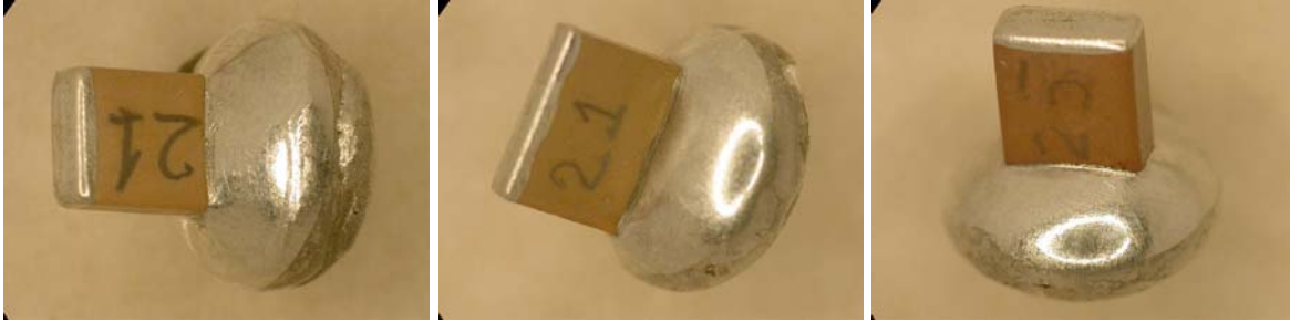
Figure 13. Examples of solder blocks attached to terminals of different types of capacitors to simulate the effect of stresses caused by excessive solder.
