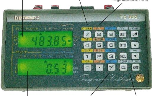
Display for measurement section (mV, V, mA, switch)
