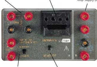
Measurement/simulation section with terminals for mA (internal or external loop supply)
