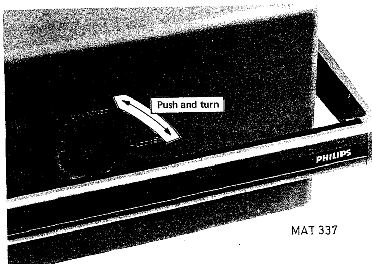
Fig. 2.2. Removing the front cover
