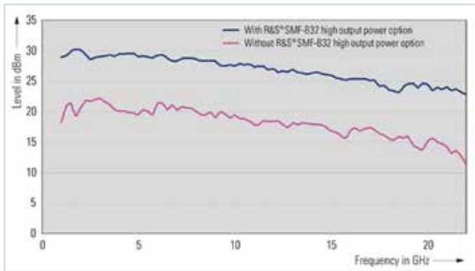
Actual maximum output power of a signal generator is often found in the products data sheet. Example of the R&S SMF with and without the high output power option in the frequency range 1 to 22 GHz.
