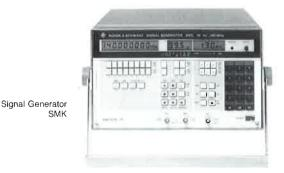
The low FM distortion (0.02%) and stereo crosstalk (down 60 dB) make the SMK ideal for measurements on top-class stereo receivers. DC coupling for external modulation sources enables FSK modulation. FM and AM can be selected independently at the same time. With FM and AM, two-tone modulation is possible for intermodulation measurements. Moreover, the SMK is suitable for swept-frequency measurements with a sweep width of up to 500 kHz (like with FM).
