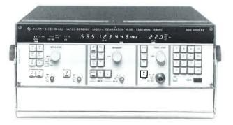
For the first time a synthesized generator with this high degree of spectral purity features also AM, FM and  $\phi$ M characteristics of maximum quality. The FM distortion of less than 0.1% and an adjacent-channel crosstalk which is down more than 56 dB permit measurements even on high-grade stereo receivers to be performed.
