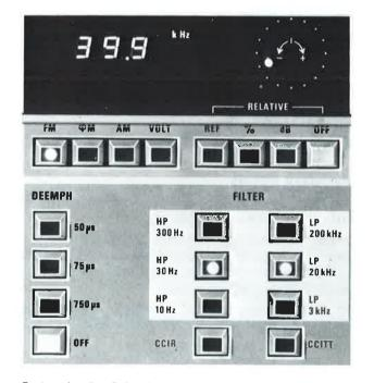
Front panel section; display of modulation measurement results and setting of operating modes
