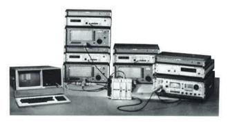
Automatic test assembly for intermodulation and crossmodulation measurements (see page 116)
