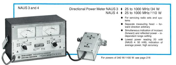
The **Directional Power Meters NAUS** are handy, easy to operate and designed for in-situ servicing of radiotelephone equipment, radio installations (up to 110 W with NAUS 4) and walkie-talkies of low output. Owing to their wide frequency and power ranges the NAUS power meters can be used over the entire radiotelephone bands for the output levels of most types of radiotelephone equipment.
