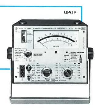
Combined with its two options the **Psophometer UPGR** complies with the relevant recommendations of CCIR, CCITT and DIN 45405. It is used for
