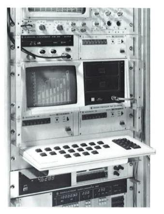
Process Controller PUC with user keyboard in 19" rack
