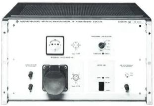
For integration in an IEC-bus system the Artificial Mains Network ESH 2-Z5 can also be remote controlled using a code converter, such as the PCW from Rohde & Schwarz.
