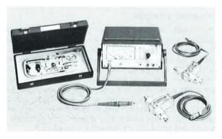
Input Impedance of RF probe. The input impedance of the RF probe is given by the input capacitance  $C_{in}$  (see to the right) and the parallel input resistance  $R_p$ , which is dependent on the test voltage (100 k $\Omega$  to 1 M $\Omega$  between 1 mV and 10 V) and, above 3 MHz, also on the frequency.
