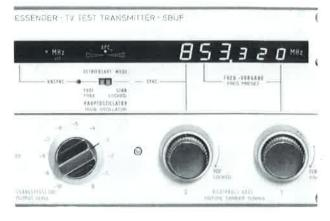
Frequency setting (bottom right) and readout (top) on Transposer Unit SBUF
