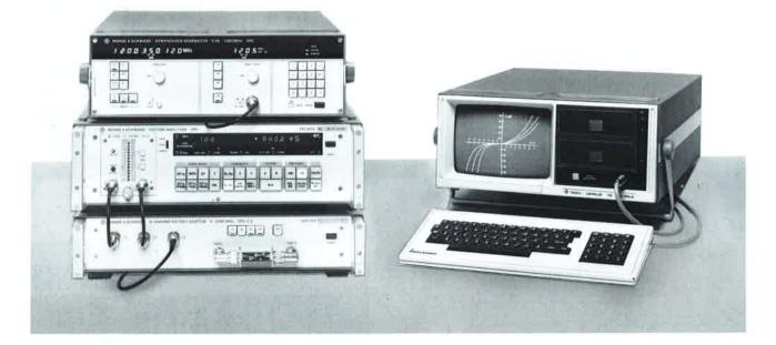
Application of IEC bus: automatic test assembly for s-parameter measurement (ZPV with S-parameter Test Adapter, XPC and Process Controller PUC)
