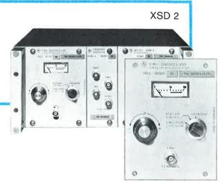
The **Crystal Oscillator XSD 2** is a particularly low-priced frequency source in the R&S standard-frequency module line. It features low aging and high short-term stability, and is very little affected by temperature variations.
