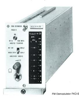
Outputs. A low-impedance output on the rear panel delivers the mono signal for monitoring and measuring purposes. The multiplex signal is available at two parallel, lowimpedance outputs on the front and rear panels. A headphones output for the L and R signals is fitted on the front panel.
