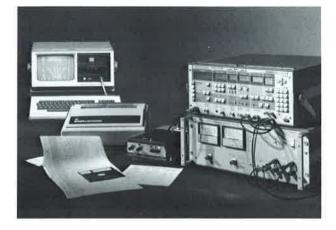
Automatic test system for AM, FM and φM transceivers
