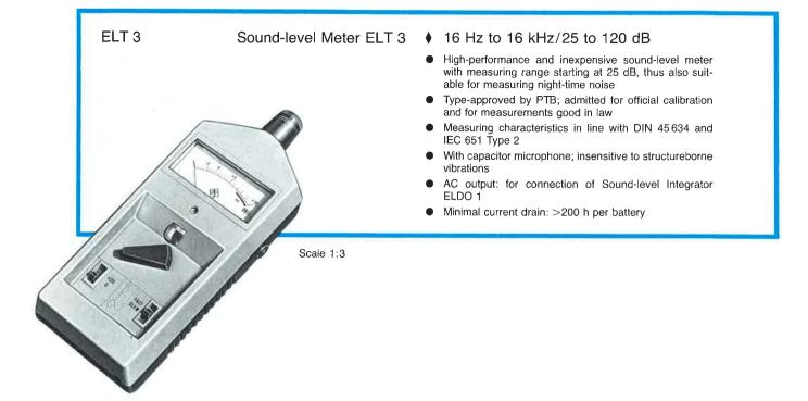
The **Sound-level Meter ELT 3** is a new and very inexpensive instrument with measuring characteristics in line with DIN 45 634 and IEC 651 Type 2. Several features, such as pickup pattern and sound-volume range, also comply with DIN 45 633, IEC 179.
