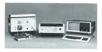
Automatic interference-voltage measurement with programmed phase-switching: Test Receiver ESH 3, Artificial Mains Network ESH 2-Z5, Process Controller PUC and Code Converter PCW
