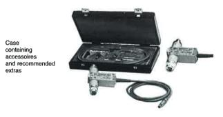
Input impedance of RF probe. The input impedance of RF probe is given by the input capacitance  $C_{in}$  (see to the right) and the parallel input resistance  $R_p$ , which is dependent on the test voltage (100 k $\Omega$  to 1 M $\Omega$  between 1 mV and 10 V) and, above 3 MHz, also on the frequency.
