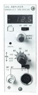
Front panel of Logarithmic Amplifier plug-in SWOB 5 E3
