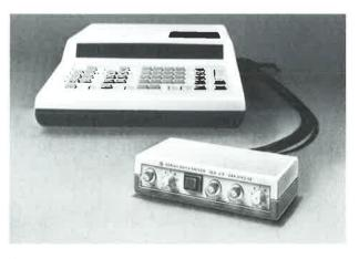
IGA with Serial Data Driver IGA-Z9 for bit-serial data generation (two Serial Data Drivers can be connected simultaneously)
