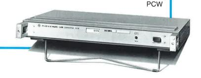
The **Code Converter PCW** is necessary if instruments designed for parallel remote control are to be programmed via the IEC bus. The PCW receives serial ASCII signals and delivers TTL levels at 44 parallel data outputs.
