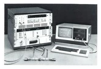
RF-component tester with test adapters for Q and capacitance measurements on chip capacitors
