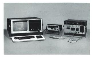
Program-controlled frequency measurement with Signal Generator SMS, Process Controller PUC and Millivoltmeter URV4
