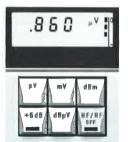
SMFP2/SMFS2 output-level display combined with readout of electronic-attenuator setting plus keys for entry and conversion of physical units
