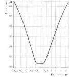
Typical filter characteristic of a PBO
