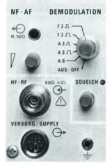
Front-panel section: demodulation and AF setting; RF input, squelch and power supply for Current Probe
