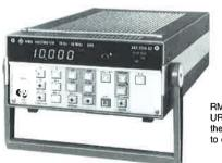
RMS Voltmeter URE; can also convert the measured values to different units
