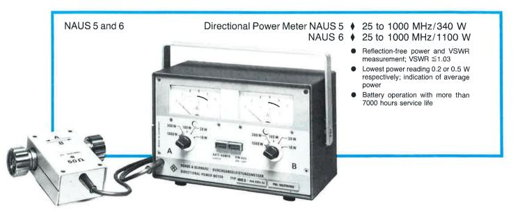
Apart from their higher power rating the **Directional Power Meters NAUS 5 and NAUS 6** are the same in design and performance as the NAUS 3 and NAUS 4 models described on pages 214, 215. Like these they consist of an **indicator** (case with carrying handle) and a separate **measuring head** which can be connected in either direction. The incident and the reflected power are indicated on separate meters in five subranges.
