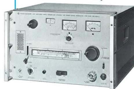
Single-stage UHF Power Signal Generator SLRD using a disc-seal triode oscillator and tunable coaxial resonantline circuits for anode and cathode. Both circuits have separate scales calibrated in MHz. The scale drives can be ganged (single-knob tuning). The whole frequency range is covered in two bands.
