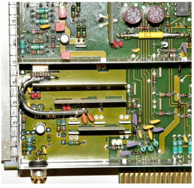
I had to put the mixer on a small PCB and attach LO and IF directly the the slot of the original mixer. IF and RF were separated by desolderung C8 and C9. RF is connected by means of a small coax cable.
