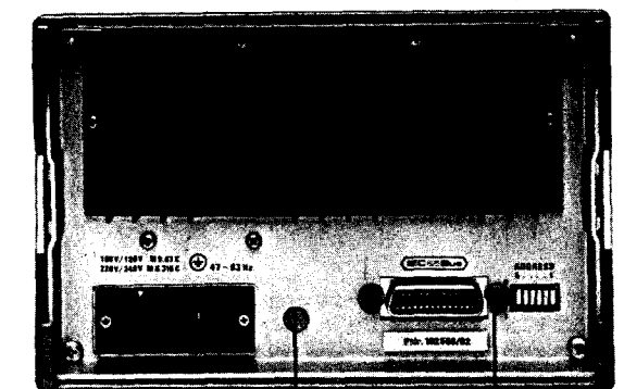
Opening for bringing out sinewave or squarewave output IEC-bus connector and address switch
