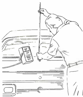
Test right at the antenna-Sensor connects between antenna cable and the CB.
