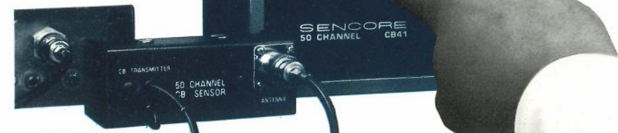
Test right at the antenna-Sensor connects between antenna cable and the CB.
