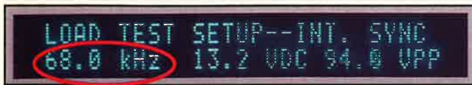
Fig. 2: For the Load Test, the HA2500 horizontal frequency control is adjusted to the monitor's top horizontal frequency.
