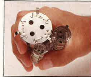
Fig. 2: Sizes of CRT's have changed dramatically over the years from the old Delta gun style to today's newest in-line. The smaller in-line gun produces much better convergence.
