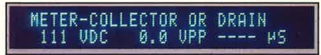
Fig. 4: The HA2500 Dynamic Test showed that the HOT was receiving B+ but wasn't switching.
