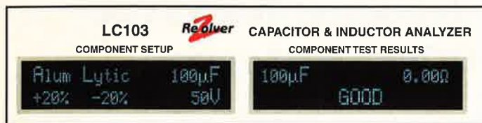
Fig. 2: The "ReZolver" clearly displays all test results and even tells you if the component is "Good" or "Bad."
