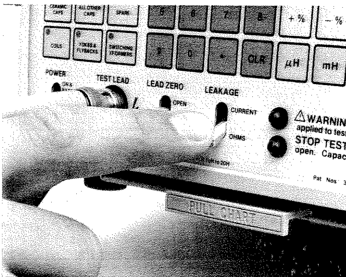
Fig. 17 — Place the LEAKAGE switch in the "ohm" position to measure leakage resistance.
