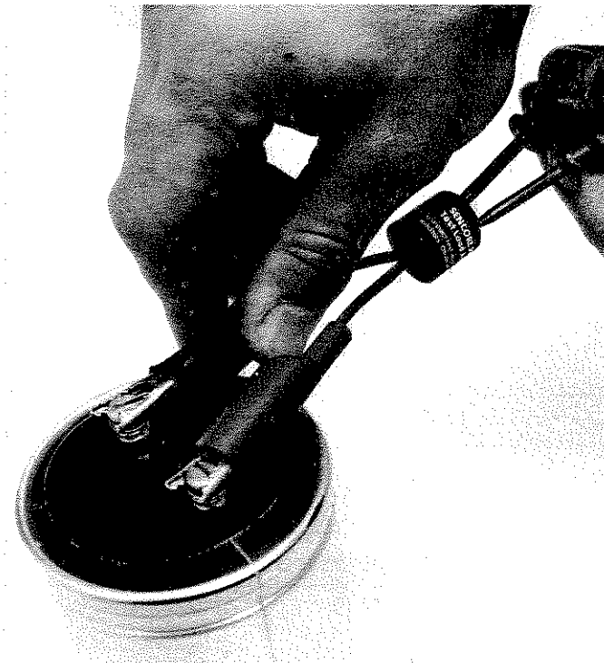
Fig. 10 - The 39G144 Test Lead Adapter allows large, screw-terminal capacitors to be connected to the LC102.
