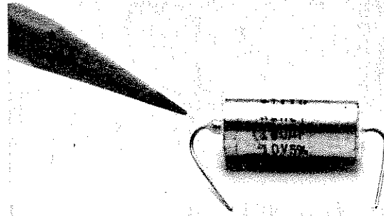
Fig. 43 — Axial lead tantalum capacitors, like the one shown here, are easily identified from axial lead aluminum electrolytics by a solder weld on one end.
