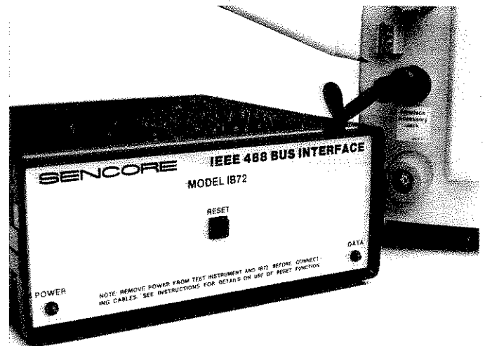
Fig. 25 - The IB72 IEEE 488 Bus Accessory interfaces the LC102 to any GPIB system for automated operation.
