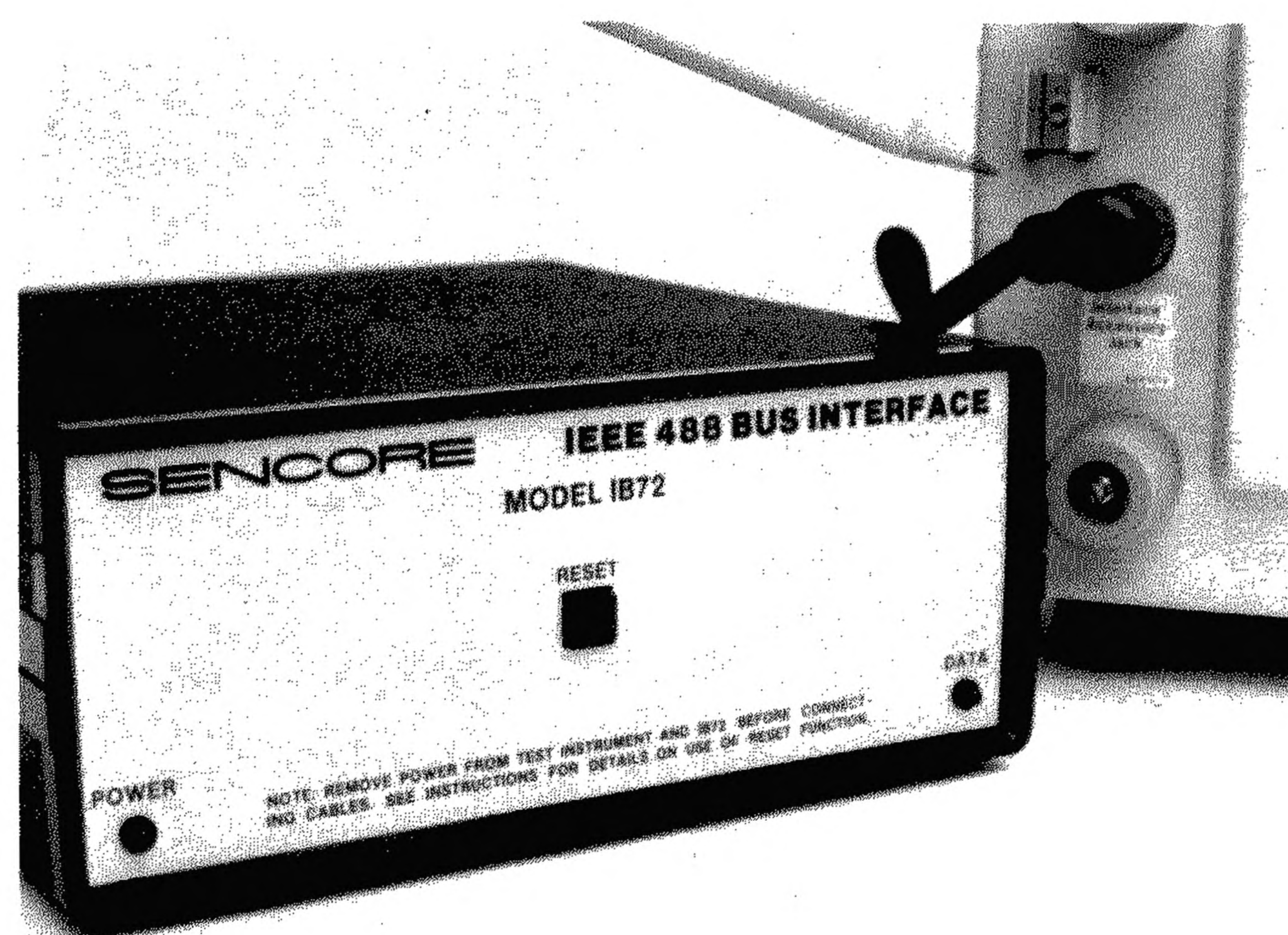
Fig. 25 - The IB72 IEEE 488 Bus Accessory interfaces the LC102 to any GPIB system for automated operation.
