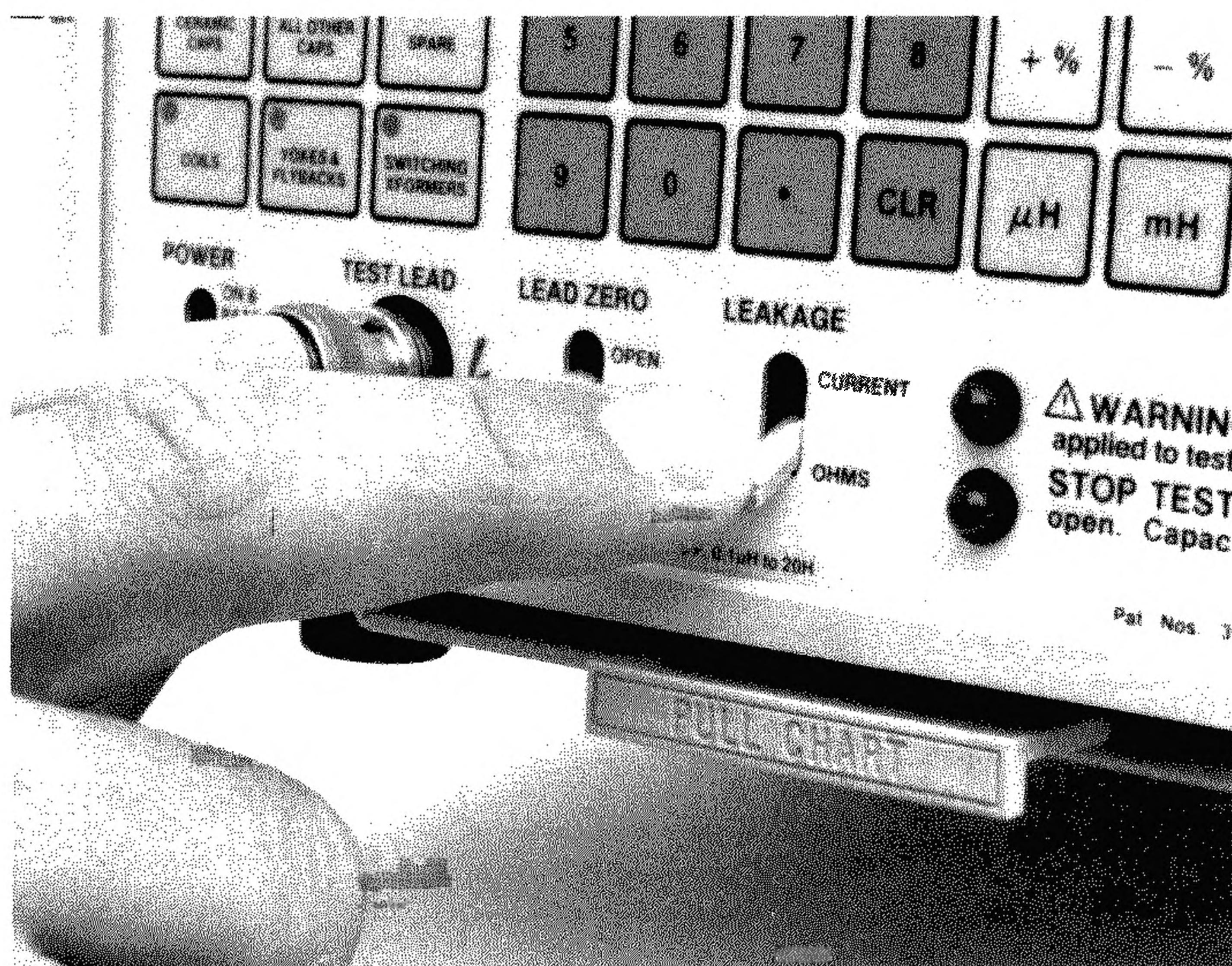
Fig. 17 — Place the LEAKAGE switch in the “ohm” position to measure leakage resistance.
