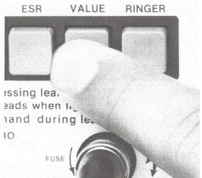
Fig. 23 — To measure inductance, connect the inductor to the test leads, depress the VALUE button and read the amount of inductance on the digital display.
