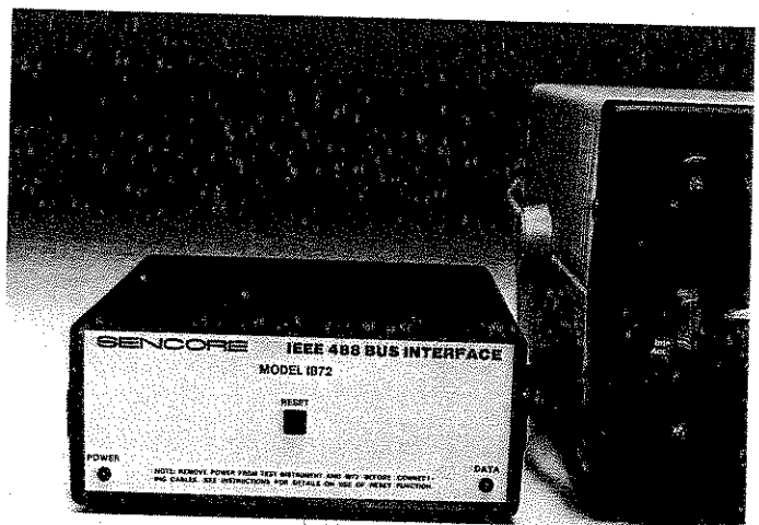
Fig. 25 - The IB72 IEEE 488 Bus Accessory interfaces the LC77 to any GPIB system for automated operation.
