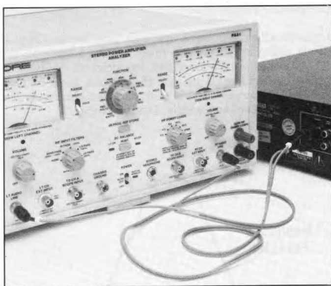
Fig. 25: For testing tuners, connect the tuner line outputs to the PA81 line inputs.
