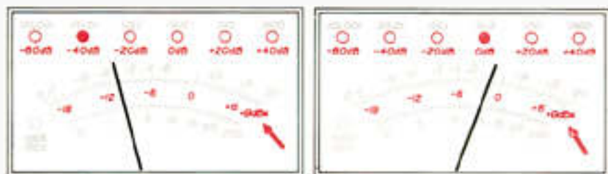
Fig. 8: Use the dBm scale to db measurements. The meters read 50 db separation; right channel is referenced to 0 db and the left channel reads 50 db.
