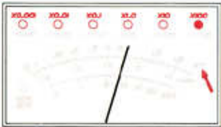
Fig. 6: Use the voltage scale to measure RMS Volts. This meter reads 60 VRMS (.6vx100).
