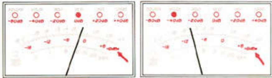
Fig. 7: Use this scale for dBm measurements. The meters read 53 dBm (-3db + -50 db)
