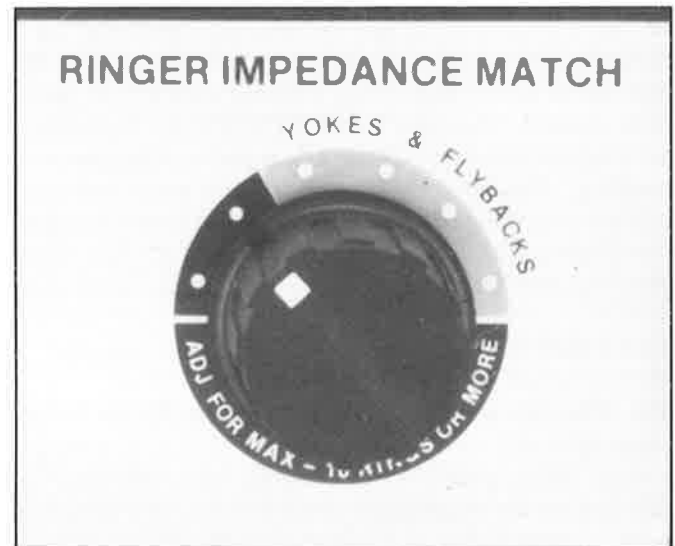
Fig. 47: The IMPEDANCE MATCHING control switches different capacitors in parallel with the coil under test.
