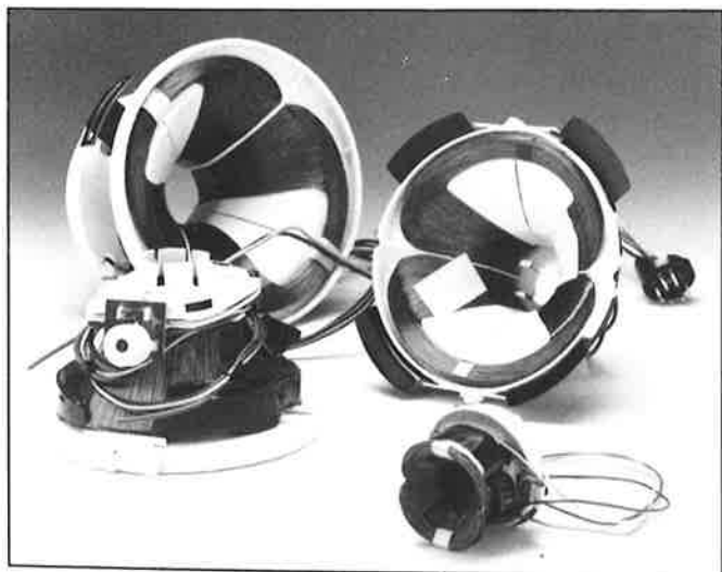
Fig. 52: The easily recognized deflection yoke can be tested accurately with the Z Meter's ringer test.
