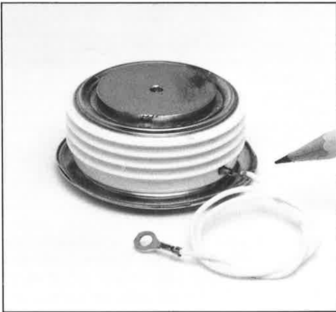
Fig. 67: The "hockey puck" SCR gets its name because of its shape.
