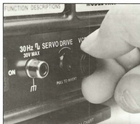
Fig. 13: The servos should respond to a phase-reversal as the VA62A's Servo Drive knob is moved to either of its two switch positions.
