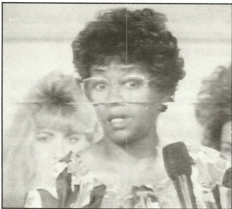
Fig. 4: A thin horizontal line at one location in the screen is not caused by a servo problem. The most likely problem is a physical scratch on the tape. If the suspect machine is scratching tapes, it will permanently place a line on every tape that passes through.
