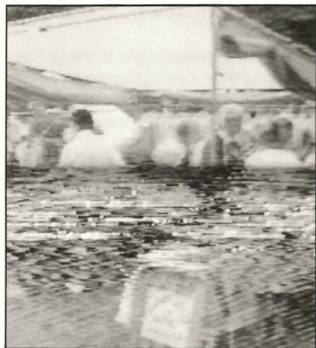
Fig. 1: Servo problems usually cause the picture to tear, or to change between clear and snowy. If the tearing remains stationary, or if the picture stays snowy all the time, the servos are not a likely cause.
