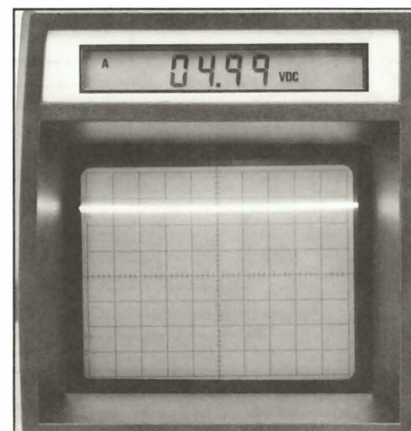
Fig. 3: The DCV feature of the SC61 Waveform Analyzer lets you quickly determine the output level of the signal being fed to the microprocessor.
