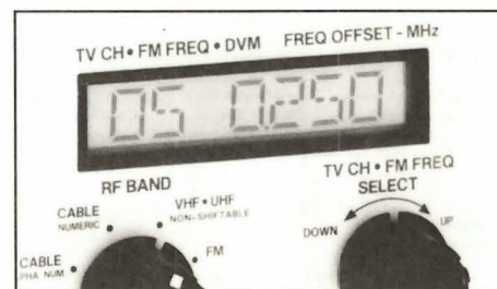
Fig. 4: The CHANNELIZERS can manually tune in 50 kHz steps to any channel from 5 to 890 MHz.
