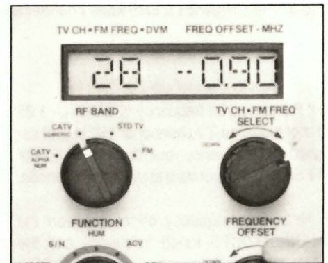
Fig. 2: The CHANNELIZERS display the frequency offset from assigned values.
