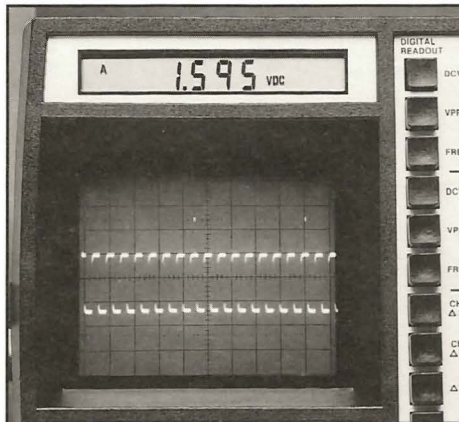
Fig. 5: Some VCRs combine the FG and PG pulse together. This is a typical example of a combined FG/PG pulse.
