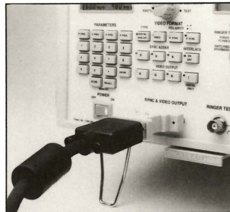
Fig. 8: Plug one end of the connector into the end of the computer monitor's cable and the other end into the CM2000's SYNC & VIDEO OUTPUT jack.
