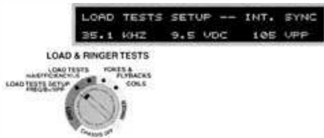
Fig. 4: Use the Load Tests Setup to set the frequency and B+ for an accurate Load Test.
