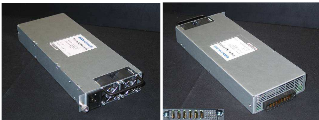
(b) Dual Output Server Power Supply: 48VDC and 5VDC
