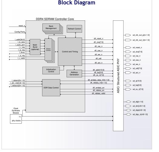
dynamic bus inversion (DBI), fine granularity refresh, additive latency, per-DRAM addressability, and temperature controlled refresh.
