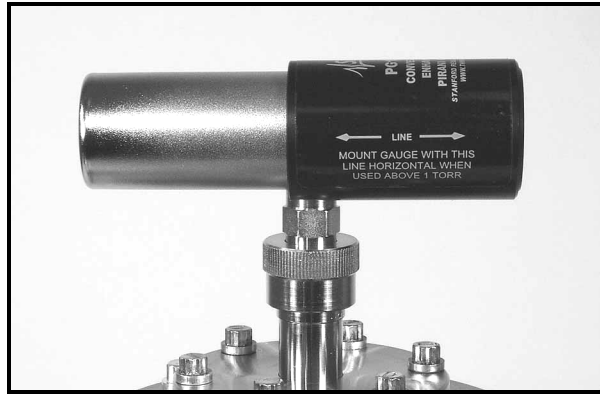
Figure H-1. PG105 Convection-Enhanced Pirani Gauge
