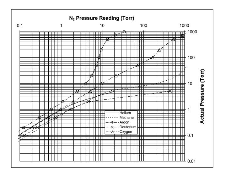
*Figure I-2. PG105 Gauge Indicated Pressure (N2 equivalent) vs. Actual Pressure Curve: 10<sup>-1</sup> to 1000 Torr. Use only when gauge axis is horizontal.*
