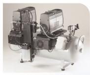
The OF1200 series of quiet, vibration-free and oil-less air compressors provides an output of 2.75 to 5.5 CFM at 120 psi. The maximum pressure is 145 psi, making the series a good choice for applications including GC, LCMS (Nitrogen generators), AA, NMR, FT-IR
