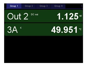
This screen displays the current values of the selected channels as numbers. The more channels that are selected, the smaller the displays are. If enough space is available, an annunciator may appear that indicates whether the sensor or heater is disconnected ("N/A"), over range ("Hi"), under range ("Lo"), if outputs are disabled ("Off"), or if an internal error has occurred ("Err").
