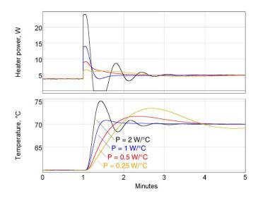
Interestingly, decreasing the proportional gain to 0.5 or 0.25 W/°C also results in more overshoot and can even cause oscillations, despite the fact that the heater response is smaller and the temperature rise slower. By reducing the proportional feedback response, we've forced the integral feedback to take more responsibility for raising the heater power — and as the next figure illustrates, the integral feedback has a greater tendency to overshoot and oscillate.
