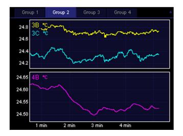
In custom plot mode, the user can manually assign each channel to a graph. Here the thermocouple inputs have been assigned to plot I and the RTD input to plot 2.
