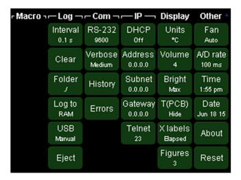
The System screen includes controls for all settings that affect the entire instrument. Time and date, Ethernet and GPIB parameters, and data logging are set up through this screen.
