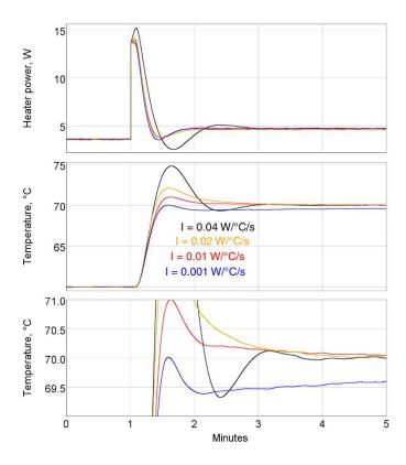
**Derivative**: derivative feedback reduces the heater output whenever the temperature is rising rapidly. In the example below, when the derivative gain D is increased from 3 to 6 W·s/°C, the amount of overshoot and oscillation decreases. The temperature rise is also a little slower, but because there is less oscillation the system stabilizes at 70°C sooner.
