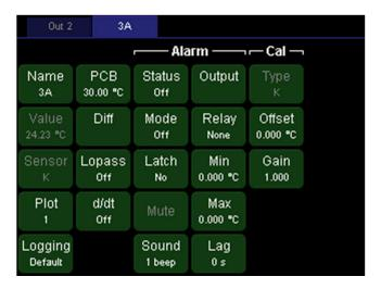
Touch the "Lopass" button to display the list of available lowpass filter time constants. To get more information about the Lopass setting, press the "Help" key, which displays a pop-up window with a brief description of whichever is currently showing on the screen. Touch the "OK" button or press the Help key again to dismiss the help window.
