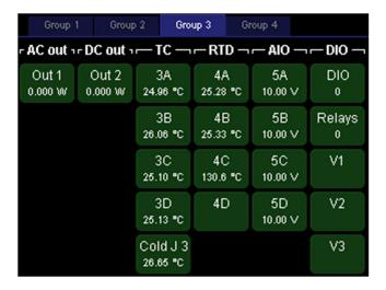
The Select screen has one column for each I/O card. The leftmost four columns are for optional I/O cards; some of these columns will be empty if fewer than four such cards are installed.
