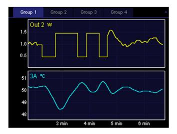
Heater power (top) and sensor temperature (bottom) during relay autotuning. Step Y is 1 W, Lag is 30 s, feedback is initially on, and the system starts with the temperature stabilized at the  $50^\circ$ setpoint. After the tuning has finished, the feedback turns on and re-stabilizes the system at  $50^\circ$ C after a few cycles of oscillation.
