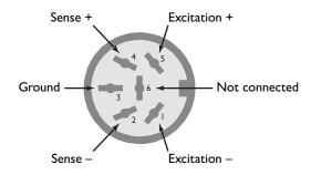
The outer shell of the plug is connected to the PTC10's chassis.
