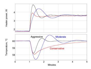
The actual behavior of your system might vary significantly from the behavior shown in these figures. In any event, the feedback gains determined by the automatic tuning algorithms should generally be regarded as only a starting point. In critical applications, the gains normally need to be manually adjusted to achieve good feedback performance.
