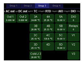
Buttons turn red if the channel's alarm is triggered; that is, if the alarm is enabled and the reading is outside of the alarm limits or no sensor is connected. The name of the channel appears in bold if the channel uses a custom calibration table.
