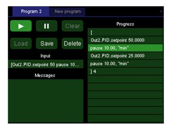
A program is a set of one or more instructions that can be used to customize the behavior of the instrument. Programs can be input over the RS-232, GPIB, USB, or Ethernet interface, from the program screen, or as a files on a USB memory device. Regardless of how a program was input, its progress can be monitored from the program screen.
