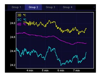
Single plot mode showing the ambient temperature measured by two thermocouples (channels 3B and 3C) and one Pt100 RTD (4B). RTDs have a much lower noise level than thermocouples.
