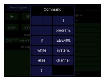
Any button with a name ending in a dot brings up a sub-menu when pressed. For example, the commands to change the feedback setpoint or alarm limits for a channel are accessed by first touching the "channel" button.
