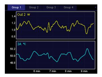
This screen shows logged data from the selected channels on one or more graphs. Press the Plot key repeatedly to cycle between the four formats described below (single, multi, custom, and ponytail).
