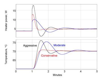
However, the results are much different if we look at how the system responds to a thermal disturbance. The next figure shows how well the system recovers when we start blowing air over the heater with a fan. The setpoint is a constant  $60^{\circ}$ C. In this case, aggressive tuning produces the best response.
