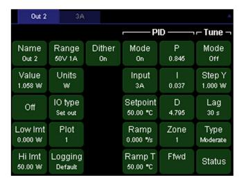
The "Channel" screen includes controls for all settings that affect individual data channels. Sensor calibration, PID feedback parameters, and alarms are all set up through this screen. Note that the layout of the screen varies depending on which channel is selected; for example, only output channels have PID controls, while only input channels have alarm controls.
