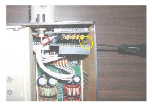
4. Install the GPIB interface board. Carfully stabilize the mating board using the screwdriver. Feel beneath the GPIB board to verify the connectors are aligned.
