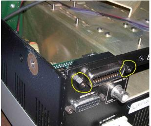
6. <u>Re-install the fan assembly</u>. Tighten the screw first, before tighening the kep-nuts.
